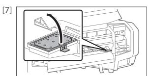
Remove the absorption material for the flushing box.
