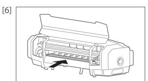
Attach the roller protective sheet.
