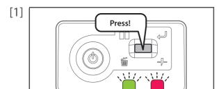
Short press the operation key on the operation panel, when the buzzer continues sounding.
