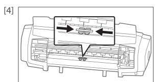
Move the paper guides to the center and place taping.
