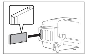
Insert cleaning cartridge to all cartridge slots.
