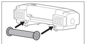
Attach the scroller to the scroller receivers.
