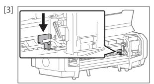
Attach the head fixing plate with screws.
