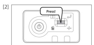
Press and hold the operation key on the operation panel for 2 seconds or more.
