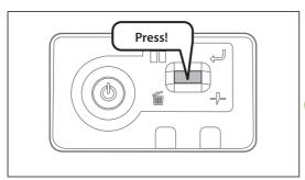
During printing, short press the operation key on the operation panel.
