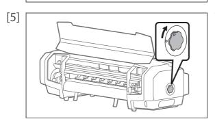
Turn the media fixing knob to release the lock.
