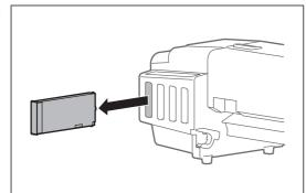
After cleaning fluid charging is done, remove all cleaning cartridges.
