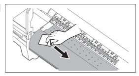
Using a soft cloth that is soaked in water and squeezed tightly, wipe dirt on the platen and media guide.
