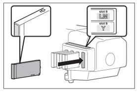
Remove the empty ink cartridge and insert the new one.
