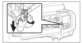
Move the cutter holder a little so that the cutter can be removed.
