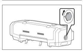
Turn the media fixing knob to release the lock.
