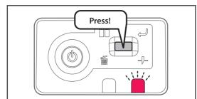
Short press the operation key on the operation panel, when the buzzer continues sounding.
