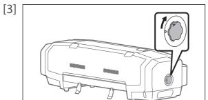
Turn the media fixing knob to release the lock.
