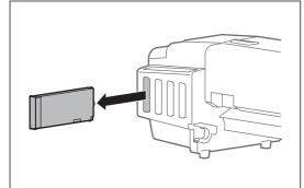
When ink cartridges are inserted to the cartridge slots, remove them all.
