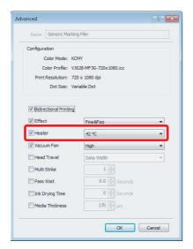
In [Heater] menu of the [Advanced] tab, enter a temperature.
