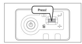
Press and hold the operation key on the operation panel for 2 seconds or more during printing.
