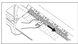
Using a soft cloth that is soaked in water and squeezed tightly, wipe dirt on the silver part of grid roller.
