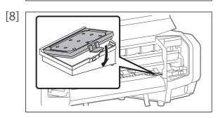
Attach new absorption material for the flushing box.
