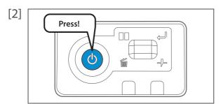
Press the power button of this product to turn the power ON.
