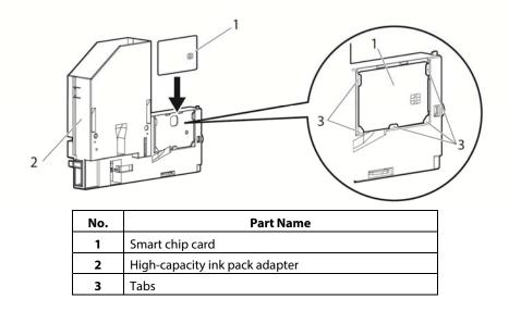
4. Make sure that smart chip card is fully inserted in place so that the card does not cover the top tabs.
