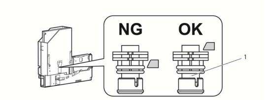
10. Use a fine-tipped tool to push out the tube connector from the left gap of the high-capacity ink pack adapter.
