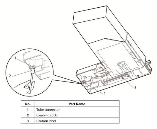
6. Install the high-capacity ink pack adapter to the printer.
