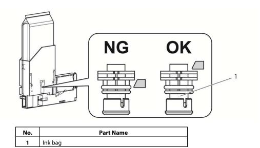
7. Make sure that the lock lever of the high-capacity ink pack adapter is back to its original position.
