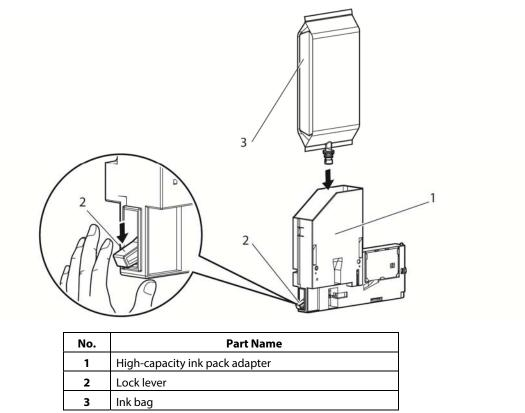
b) Confirm ink bag is fully seated by checking the lock mechanism is at the top of the ink delivery neck through the observation window, see proper placement in image below.
